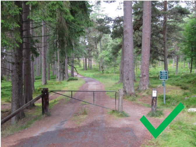
Where livestock control isn't an issue, leaving a gap at least 1.5m clear passable width alongside a vehicle barrier or locked gate is the simplest solution and maintains access for all types of legitimate recreational access.
